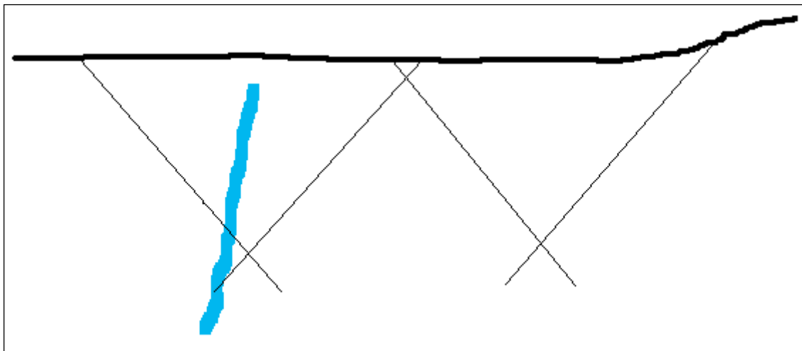
Figure 10-2: Illustration of an RC drill fence
