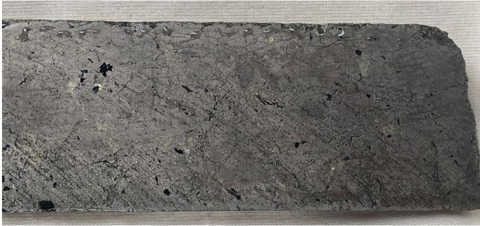
Massive sulphide with coarse pentlandite (Ni-sulphide)
